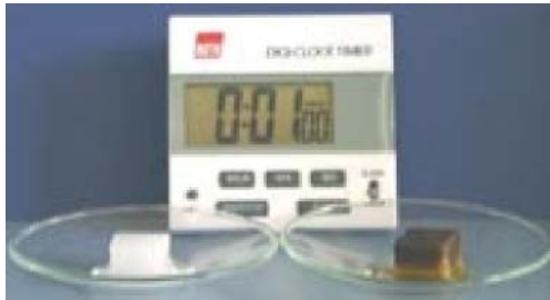
Picture 1: Effect of 20% dilute sulfuric acid (left) and concentrated sulfuric acid (right) on a sugar cube after one minute; already after a few seconds, a yellowish coloration is visible for the concentrated sulfuric acid, which rapidly becomes brown and then goes to a black coloration.
