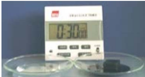
Picture 2 Effect of 20% dilute sulfuric acid (left) and concentrated sulfuric acid (right) on a sugar cube after 30 minutes; already after a few minutes, the sugar cube in the concentrated sulfuric acid is completely carbonized unlike the sugar cube in the dilute sulfuric acid which only dissolves.
